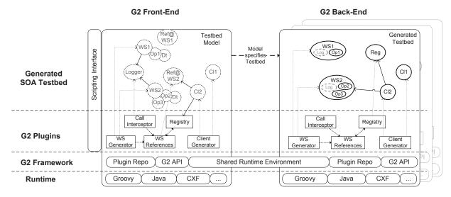
Fig. 2. Genesis2 architecture: infrastructure, plugins, and generated elements
