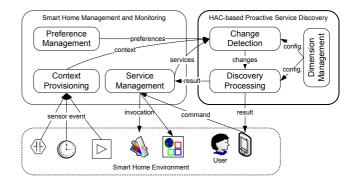
Figure 4: System architecture
