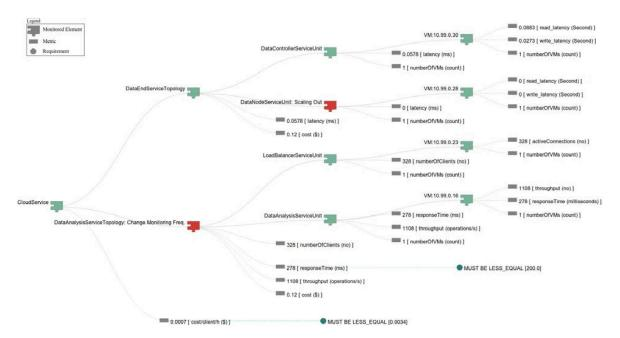
Fig. 6. Elasticity space monitoring integrated with control, deployment and testing events/metrics
