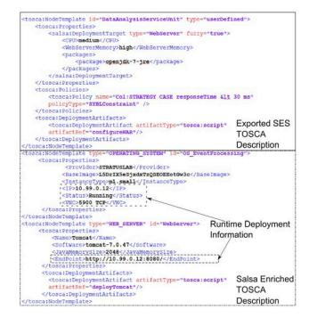
Fig. 5. Examples of SES structure, deployment and runtime description
